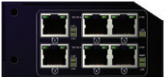
6 - 10/100 Mbit Copper RJ45 Ports
